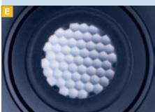
Fly-eye lens for homogeneous fluorescence illumination
