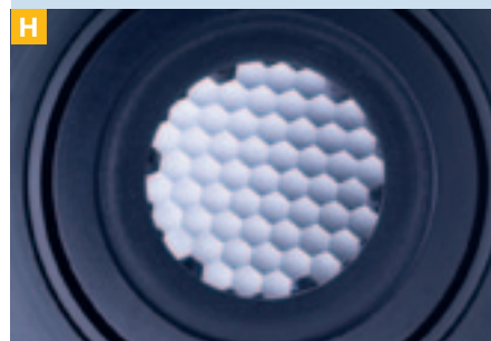
Fly-eye lens for homogeneous fluorescence illumination
